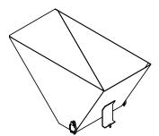
A feed hopper with a capacity of 5 kg can be mounted on the deawner. This way, the sample cleaner can be used for larger sample quantities, e.g. for seed cleaning for trial lots.
