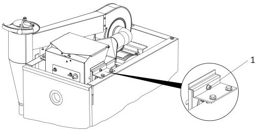
Figure 19: Screws at the filling container
