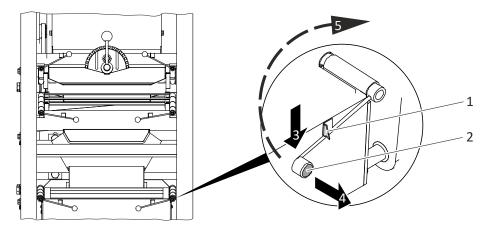
Figure 13: Tension springs on sieving tray
