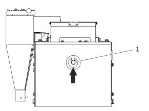
Figure 11: Locking lever for deawner bottom
