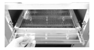
Figure 18: Grading sieve - mounting position
