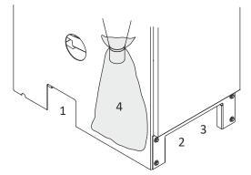
Figure 10: Placing the collection pans and the dust collection bag
