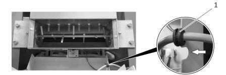
Figure 20: Rubber bush at the filling container
