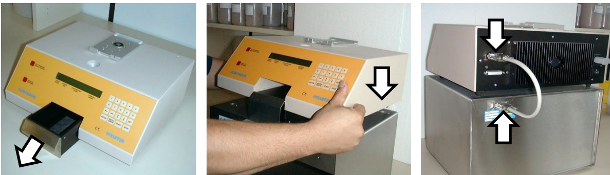
Figure 9: Put on CONTADOR and connect with CONTAFILL
