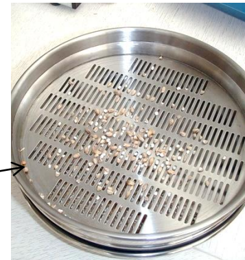
Figure 22: Mass C on hand-held sieve
