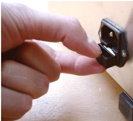
Figure 46: Renewal of the internal fuse
