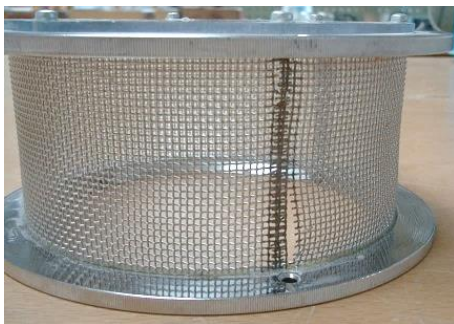
Figure 25: Damaged sieve drum
