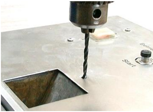
Figure 32: Drilling out rivets
