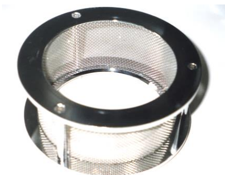
Figure 19: Putting the sieve drum down flat
