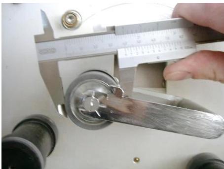
Figure 23: Checking the pressure roll diameter
