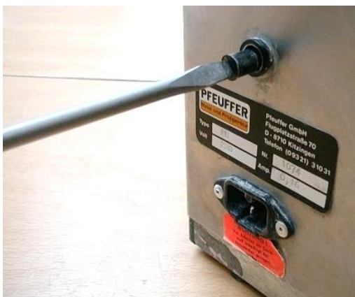
Figure 47: Renewal of the internal fuse in older devices
