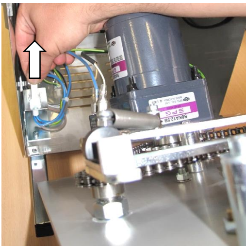
Figure 33: Disconnecting the motor plug
