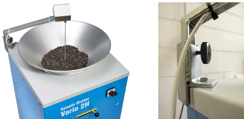
Figure 8: Agitator and fixing the holder to the cover
